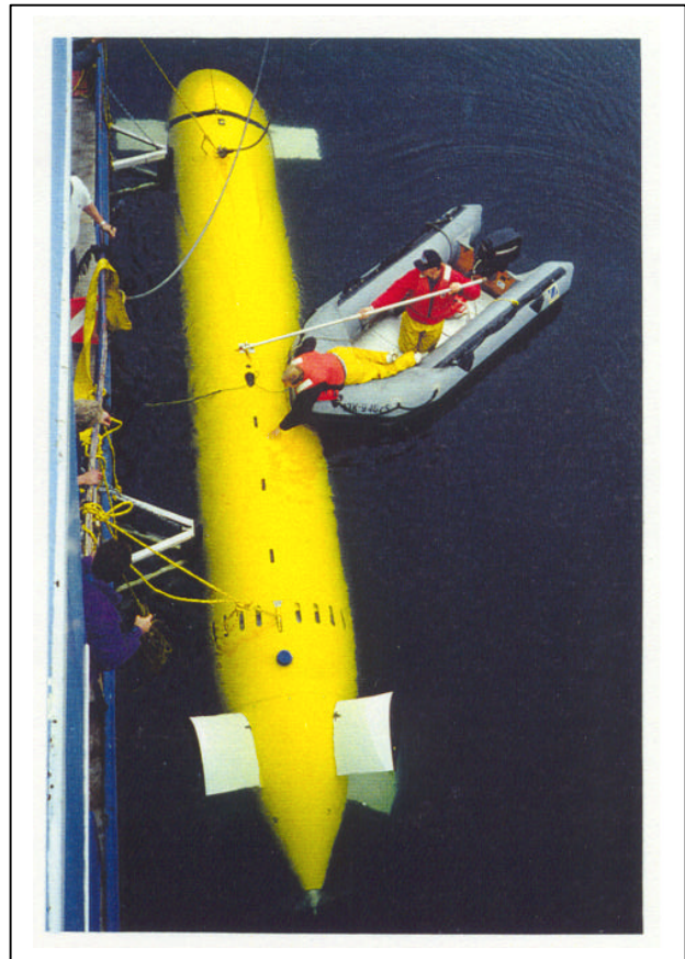
ISE's Theseus AUV (right) and schematic (below)
