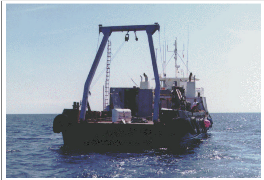
Stern launch configuration for the LLS towfish
