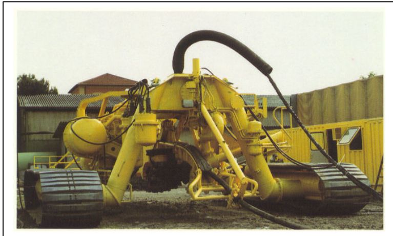
Tecnomare's TM 402-C Cable Trenching Vehicle (left) and Concept of Operation (below)
